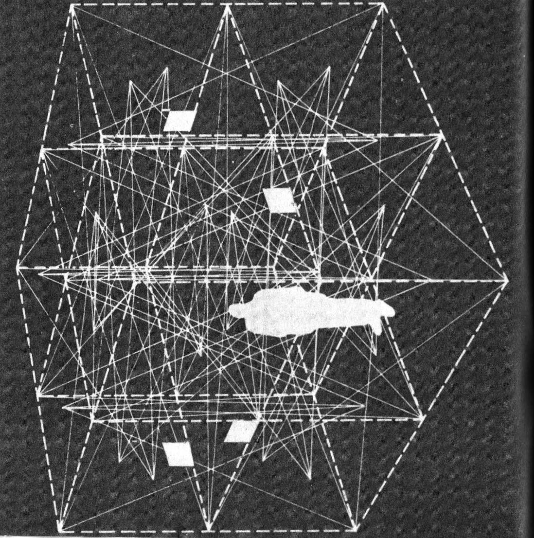
This projection diagram for the KNOWLEDGE BOX shows the four 6' projection modules on each of the six faces of the 12' chamber.
