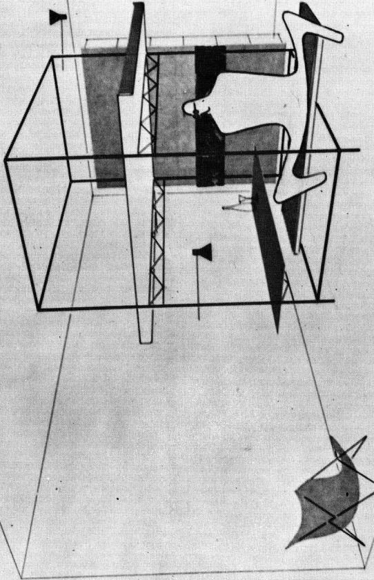
LIVING STRUCTURES may be built of all kinds of materials from steel tubing to bamboo. This one is of aluminum tubing with welded trusses supporting the bed and table. The cooking shelves are behind the panel which has a vertical pass through opening.
