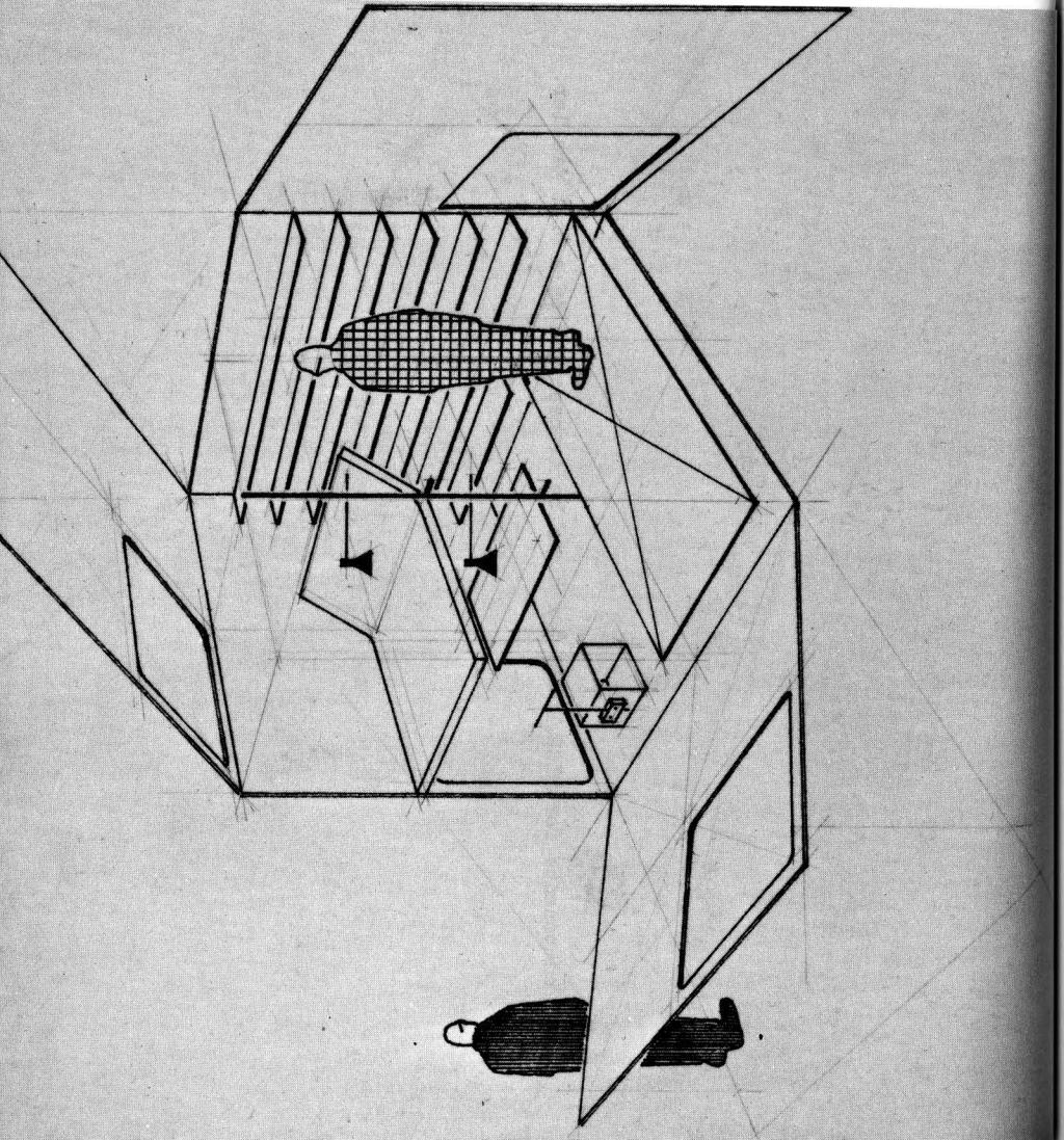
The MICROHOUSE 8 x 8 has an elevated sleeping surface with skylite over it and sitting-eating area beneath. Hygiene and bathing facilities are under the raised floor with cooking and storage shelves on the back wall.
