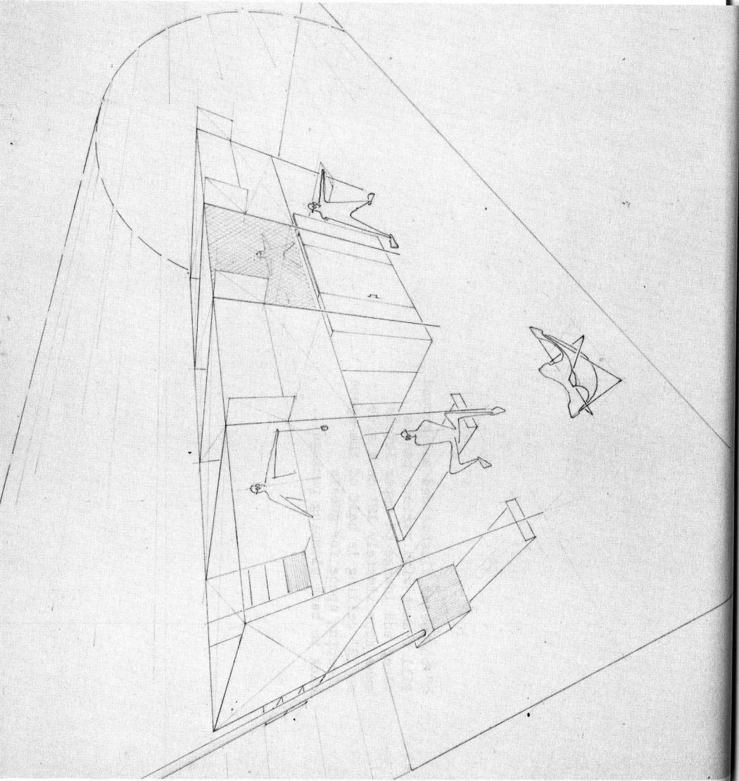
This house is one of the earliest embodying the principle of separation of weatherproofing from interior structure. The sheltering vault may be concrete or plastic. This idea makes possible an entirely new freedom and clarity in the house.
